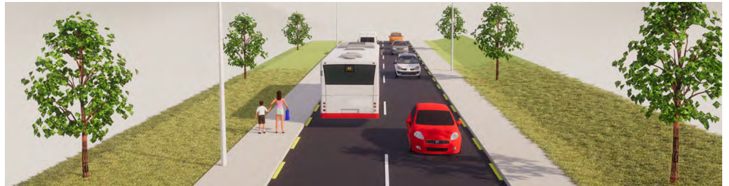
Figure NTS-12: Single Carriageway (With Footway)
