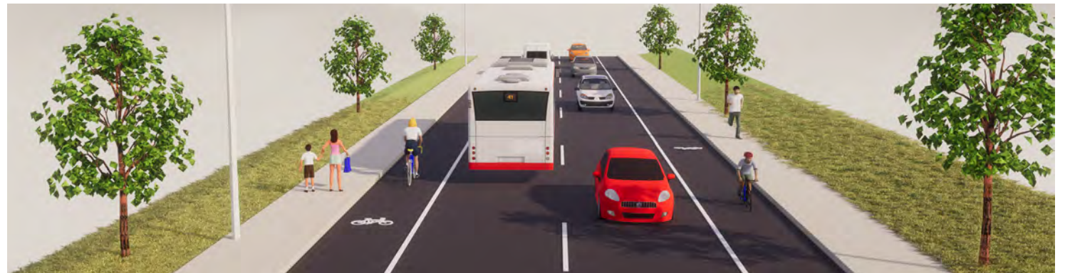
Figure NTS-13: Single Carriageway (With Footway & Cycleway)
